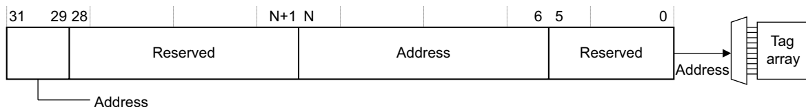
Figure 3-86 L2 tag array read operation format
