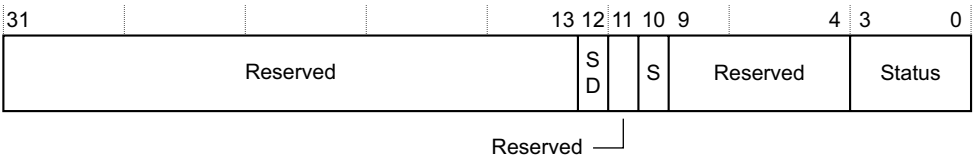
Figure 3-31 Instruction Fault Status Register format
