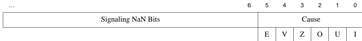
Figure 14-34 Output Format for Faulting Elements when NX is Set
